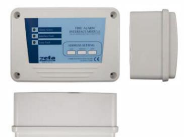
The Pulsor addressable input unit (ZIU-PLR) is used to interface external equipment which has a volt free normally open relay output to any Pulsor addressable fire alarm system. The input is monitored with a 47K end of line resistor. The unit has a built in loop short circuit isolator to help keep the unit operational in the event of a problem on the addressable loop wiring. The unit has internal LED indications for loop isolator active, fault on input and alarm (panel controlled).
